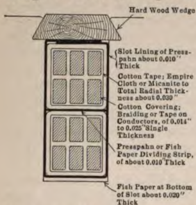
FIG. 32.—Insulation of conductors in slot.
